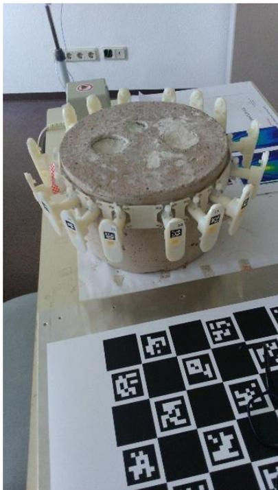
Scan belt with maximum 64 transducers and fast wireless position acquisition
