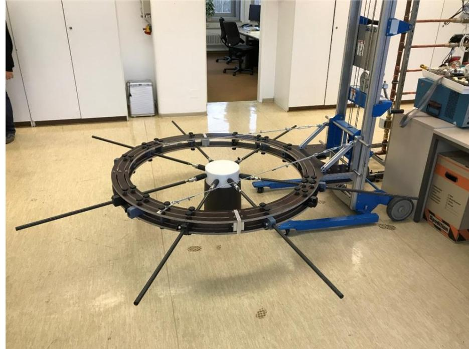
Scan ring with maximum 24 transducers and automatic position acquisition
