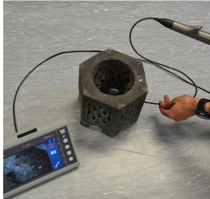
Recording of surface with scanner; voids with endoscope
