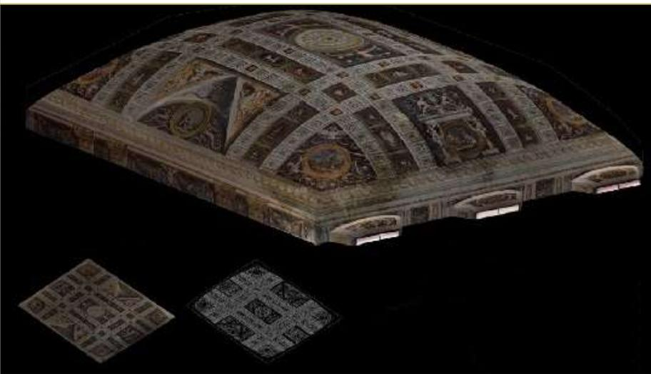
3 'similar' construction solutions obtained on the common 'cloister' typology. some details of the 2 deviations: the Manfredini Hall, Cloister - to -Trompe solution (centre), and the Stair Hall, Cloister-to-Dome-to Trompe corners (below); Magio Grasselli Palace.
