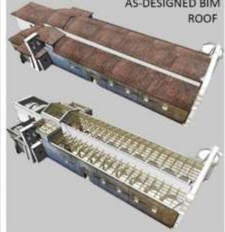
AS-DESIGNED ROOF internal view
